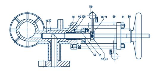
Another SchuF innovation, the 30T, allows the valve to be installed horizontally. This enables the operator to take a vertical sample without having to operate the valve under the pipe – a potentially dangerous situation should hot polymer splash or spill while the sample is being taken.
