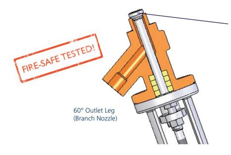
Metal to Metal Seal Disc Opens into the Process Medium
