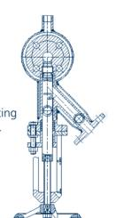
Max. Temperature: PTFE Packing Rings: 260°C Graphite Packing Rings: 550°C
